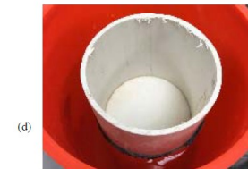
Figure 2. Flow through column for coefficient of retardation measurement setup.
